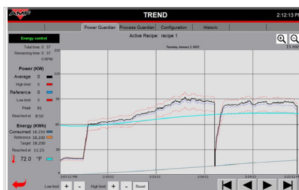
Mixer Guardian Power Monitoring System
